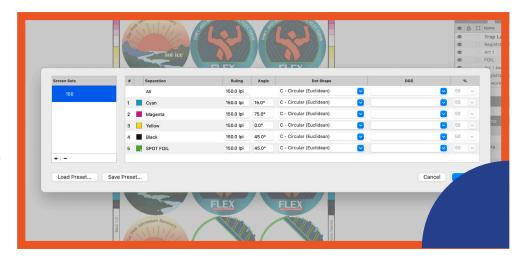
**Trapping:** Using the trapping tool to set the trapping to the correct settings (pictured on the right). After this, we used the automation engine to create our color separations and sent them to the Esko CDI spark 2530 imager merger program.
