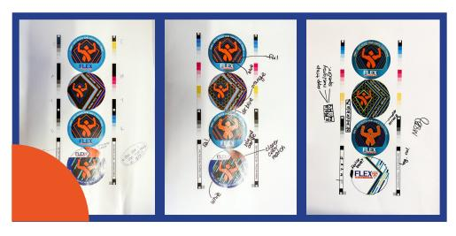
Final Proof: I printed my proofs using the Konica Minolta. It took three proofs and design adjustments to reach the final proof (pictured on the right). After the designs where signed off on, the final adjustments listed on the proof were made in illustrator.
