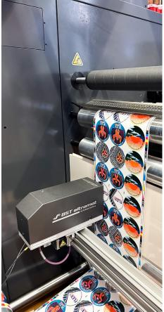
Quality Control: Using the jm heaford plate mounter and nilpeter quality control systems we ensured that are plates and prints were in registration throughout the platemounting and printing process.
